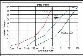
The speed of cure will depend on ambient temperature, low temperatures will slow the cure times and higher temperatures will speed the cure.
